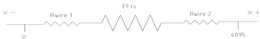
Figure1 (b): Equivalent Circuit of 4-wire Touch Screen
